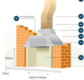
Ventilation required for nominal 450mm wide finished fire opening 18,500mm² permanently open free air space provided by 2 No. 215 x 215mm Rectangular Hole Air Bricks, list no. 374, each providing 10,250mm² free air space and 2 No. 215 x 215mm Cavity Wall Bridging Ducts, list no. 402.
