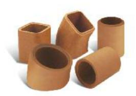
B2 N2 liners are made from natural red clays and are distinguishable from liners conforming to class A1 N2 which are made from a lighter density, buff, fireclay. This enables the A1 N2 liner to withstand the severe temperature fluctuations in the soot fire resistance test.
